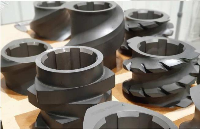
For applications subject to high wear GTS offers screws wear protection on the running surface of the screw flights, manufactured by PTA process or by Laser Technology. This can be combined with an excellent chrome-coating or high-speed TC-coating inside the screw channels. For customer-specific requests, a customized solution is always economical.
